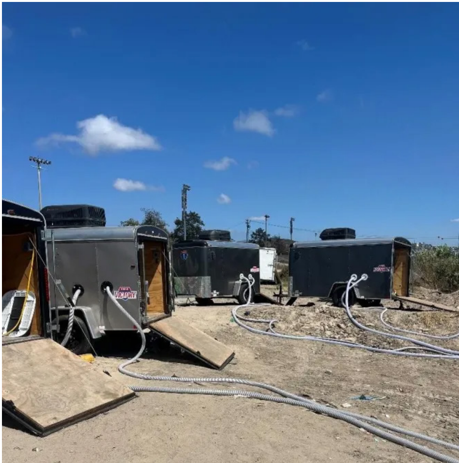
Ozone nanobubble equipment treats Mexican sewage along the Tijuana River in San Ysidro (2025). Photo provided by the U.S. International Boundary and Water Commission.
