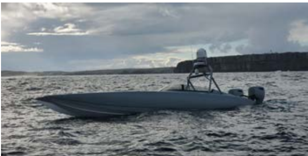
A T-38 Devil Ray unmanned surface vehicle. Photo courtesy of Dave Meron.
