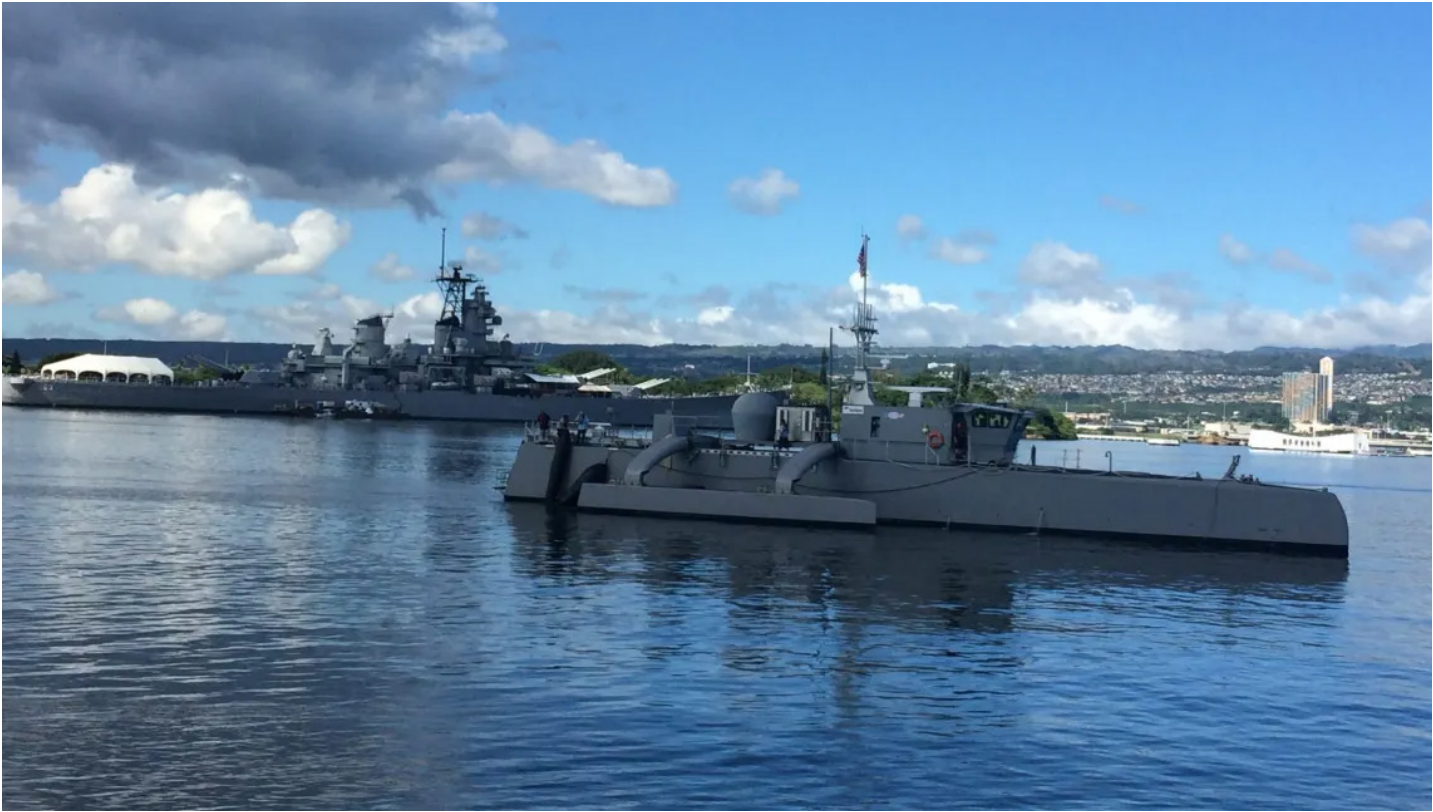
The Sea Hunter, seen in this 2018 photo, is an unmanned sea surface vehicle developed in partnership between the Office of Naval Research (ONR) and the Defense Advanced Research Projects Agency (DARPA). The Sea Hunter is part of ONR's Medium Displacement Unmanned Surface Vehicle (MDUSV) project. Photo courtesy of the U.S. Navy.
